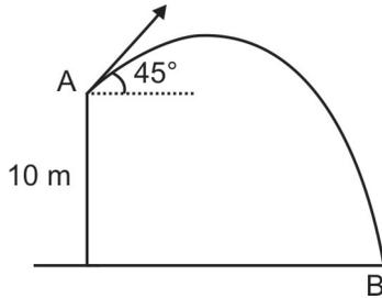
Total mechanical energy at A = Total mechanical energy at B
