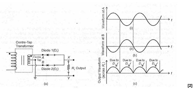
Consider the input voltage to A with respect to the centre tap at any instant is positive then at that instant, voltage at B will be negative and vice-versa.
