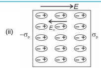
When a dielectric slab is inserted between the charged plates of a capacitor, due to polarization of molecules of dielectric slab an internal electric field is generated in slab in the direction opposite to that of between the plates of capacitor. Hence, net electric field between the plates of capacitor decreases.
