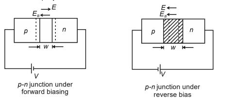
In forward biasing positive terminal of battery is connected to the p side and negative terminal to n side. Due which p-n junction width becomes slightly narrower.
