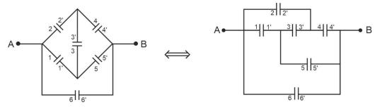
In the above circuit diagram, we can remove capacitor with plate number 33' by applying Wheatstone bridge principle.
