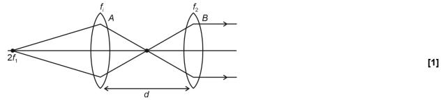
Emerging ray will be parallel to principal axis if image of lens A is formed at the focus of lens B
