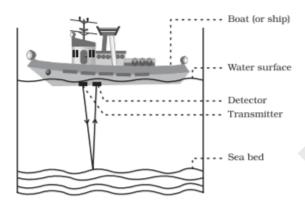
The transmitter produces and transmits ultrasonic waves. These waves travel through water and after striking the object on the seabed, get reflected back and are sensed by the detector. The detector converts the ultrasonic waves into electrical signals which are appropriately interpreted. The distance of the object that reflected the sound wave can be calculated by knowing the speed of sound in water and the time interval between the transmission and reception of the ultrasound.
