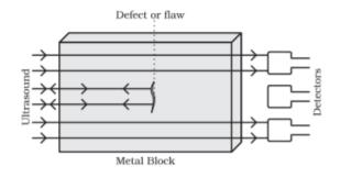
Ultrasound is reflected back from the defective locations inside a metal block.
