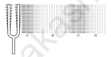
Here C is for Compression and R is for Rarefaction.
