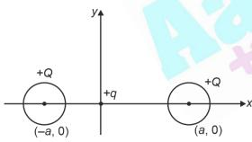
**Case-I:** If small ball will displaced along *x*-axis, it will always tend to move at point of minimum potential energy that is origin.
